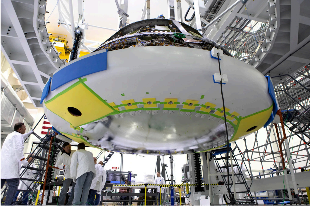
Figure 11: Technicians working on an Orion crew module heat shield during spacecraft assembly. The Artemis II heat shield consists of 186 pre-machined AVCOAT blocks bonded onto a carbon fiber substrate, covering the full 16.5-foot diameter base of the capsule. Credit: NASA/Lockheed Martin.
