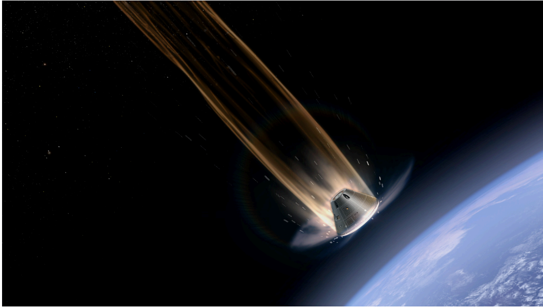
Figure 6: Artist's concept of Orion during atmospheric reentry, surrounded by ionized plasma generated by the hypersonic shockwave ahead of the heat shield. Published figures for the heat shield surface range from about 3,000°F to nearly 5,000°F (2,760°C); the shock layer itself is far hotter. Credit: NASA.
