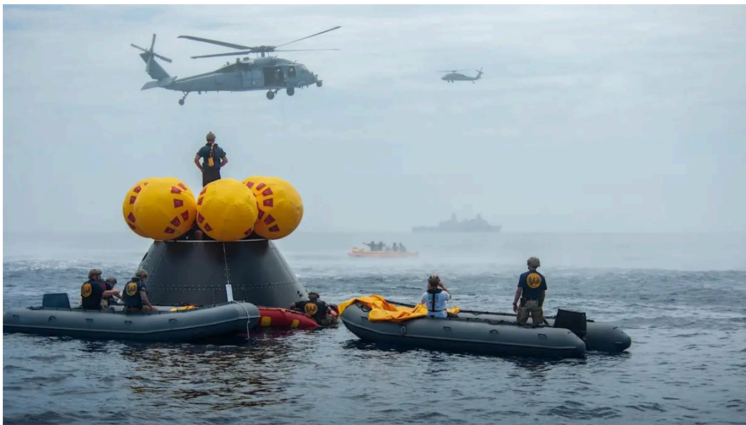
Figure 15: Navy divers and recovery personnel securing the Orion crew module following splashdown during an Underway Recovery Test (URT). The recovery choreography involves four helicopters, rigid-hull inflatable boats, and open-water Navy divers who enter the water after splashdown. The USS John P. Murtha served as the primary recovery vessel for Artemis II. Credit: NASA.
