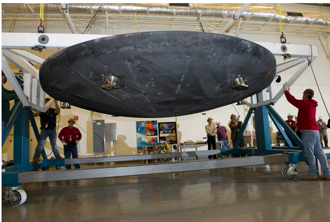
Figure 9: An Orion heat shield being lifted during ground processing. After Artemis I, post-flight inspection found unexpected loss of charred AVCOAT at more than 100 locations: the char, which is designed to erode smoothly, instead cracked and broke away after gas built up inside it during the skip entry. This anomaly directly drove the decision to shorten the skip for Artemis II. Credit: NASA.
